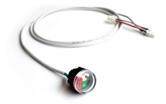
With a built-in PSW charger the LEDs are not always visible. An external LED can be used in this case. This option requires no extra installation procedure. All that is needed is a **simple plug & play connection**. The LED has 3 different statuses: 'charging', 'charging done', 'deep discharging'. If required one can even use the standard built-in relay in the PSW. This can be used to switch off a consumer.
