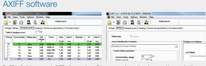
The EDrive Fortis has a separate AXIFF software package. This program can be used to make a very wide range of settings. One can configure **individual charging curves** for example.
